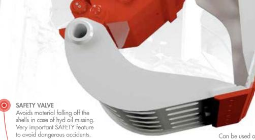
BOLT ON REPLACEABLE CUTTING BLADES
